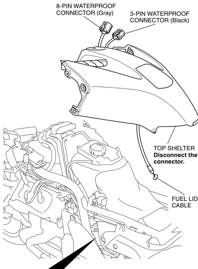
Pull outward slightly on the left rear cowl until the boss is released. Disconnect the fuel lid cable as shown.
