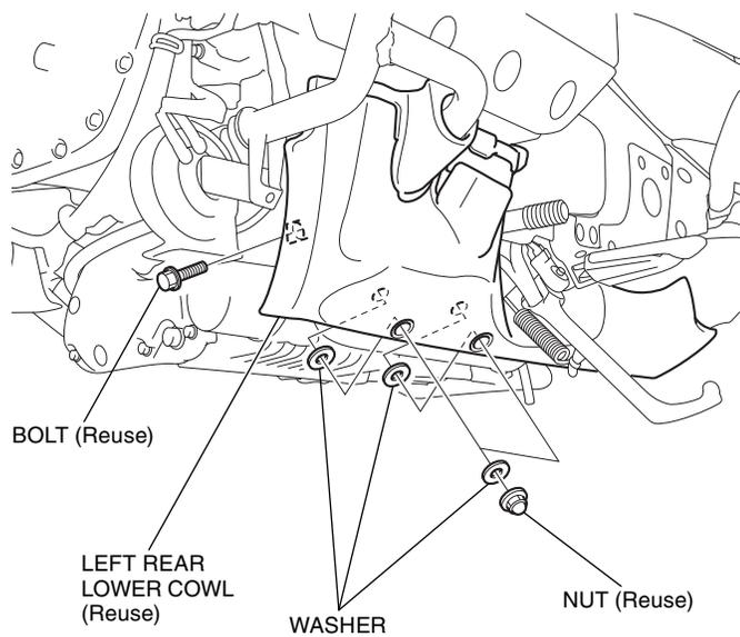
9. Install the motorcycle's parts in the reverse order of removal.
