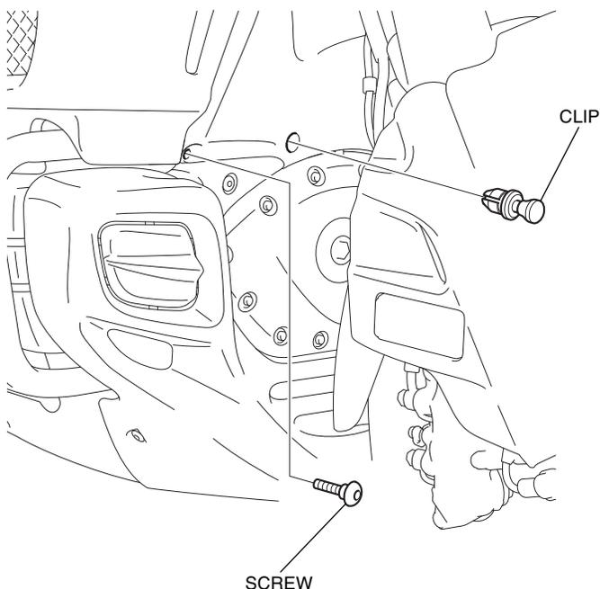
2. Remove the front lower cowl and the front upper cowl as shown.
