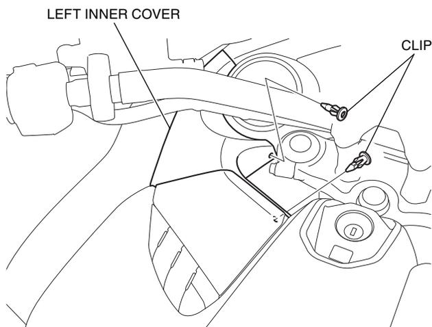
2. Remove the left inner cover, and then disconnect the negative (-) battery cable.
