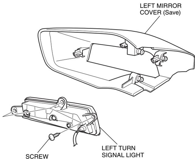
6. Install the left turn signal light into the accessory left mirror cover in reverse order of the removal.
