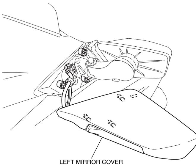
4. Remove the left turn signal light harness as shown.
