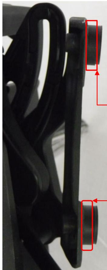
Plastic washers location (under the flange of the original insert)
