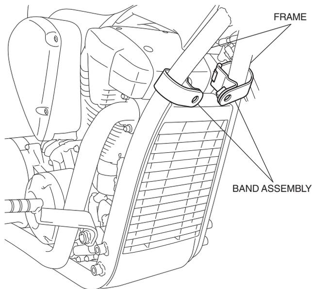
5. Loosely install the engine guard.
