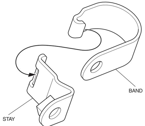
4. Loosely install the assembled bands as shown.
