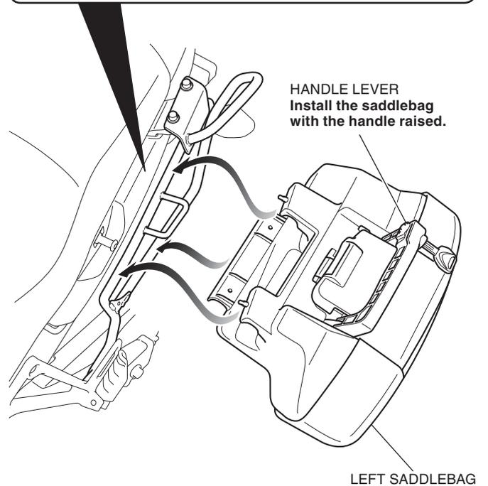
3. Lower the handle lever and lock the left saddlebag by turning the key counterclockwise as shown.
