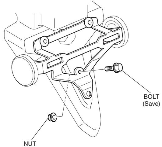
2. Remove the reflector as shown.
