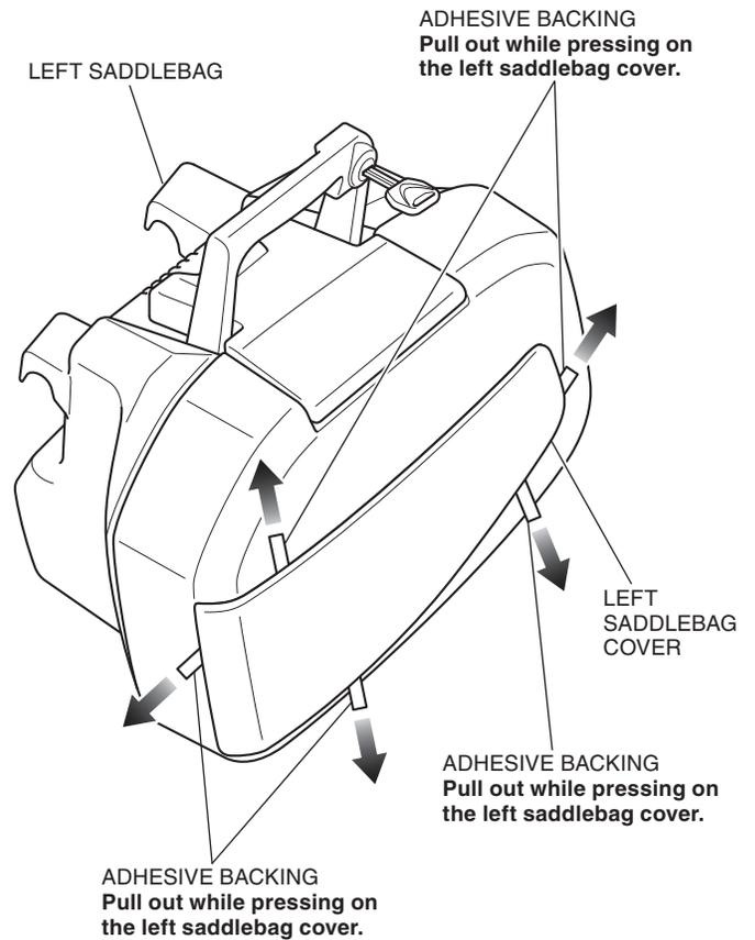
5. Apply adequate pressure to the attached left saddlebag cover.
