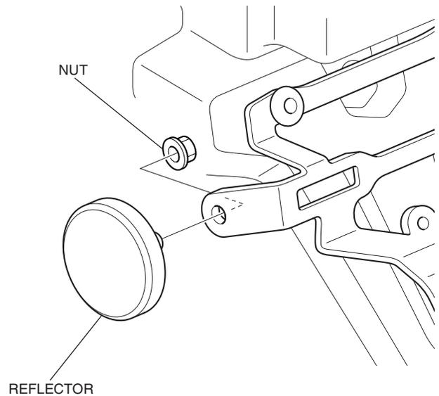
3. Install the reflector stay as shown.
