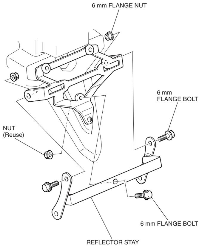
4. Install the reflector as shown.
