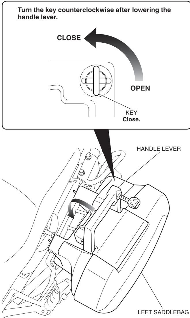
4. Remove the key. Be sure that the handle lever cannot be released and the left saddlebag is installed securely.
