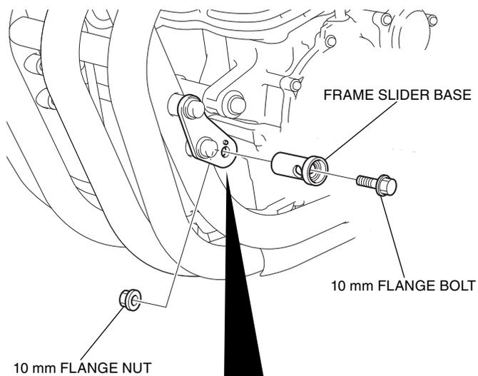
**Align the hole of the frame slider base with the projection of the left frame slider plate as shown.**
