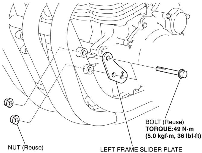
3. Install the engine guard base as shown.
