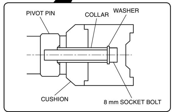
5. Install the frame slider cap as shown.
