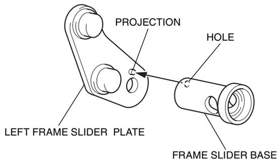
4. Install the frame slider body as shown.
