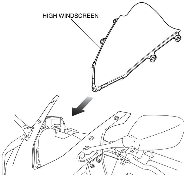
15. Install the parts as shown.
