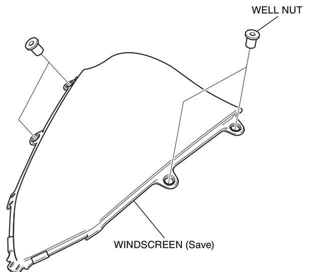
13. Install the well nuts as shown.
