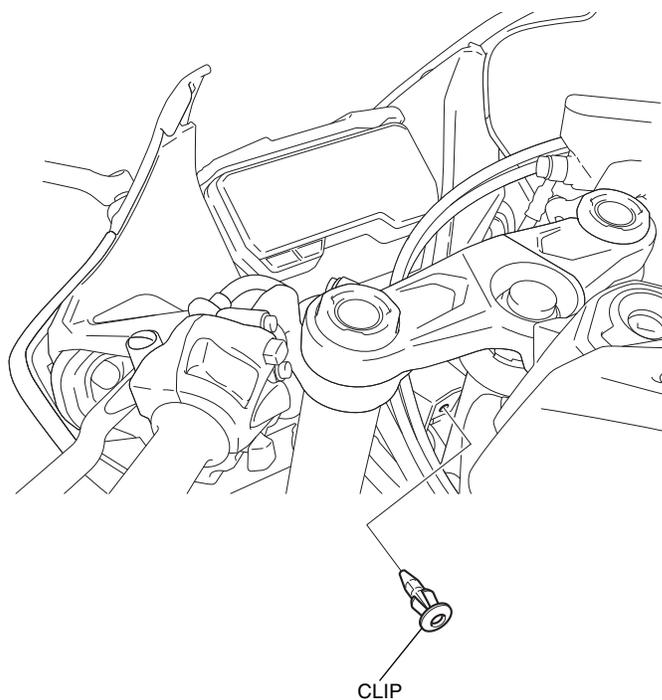
6. Remove the meter as shown.
