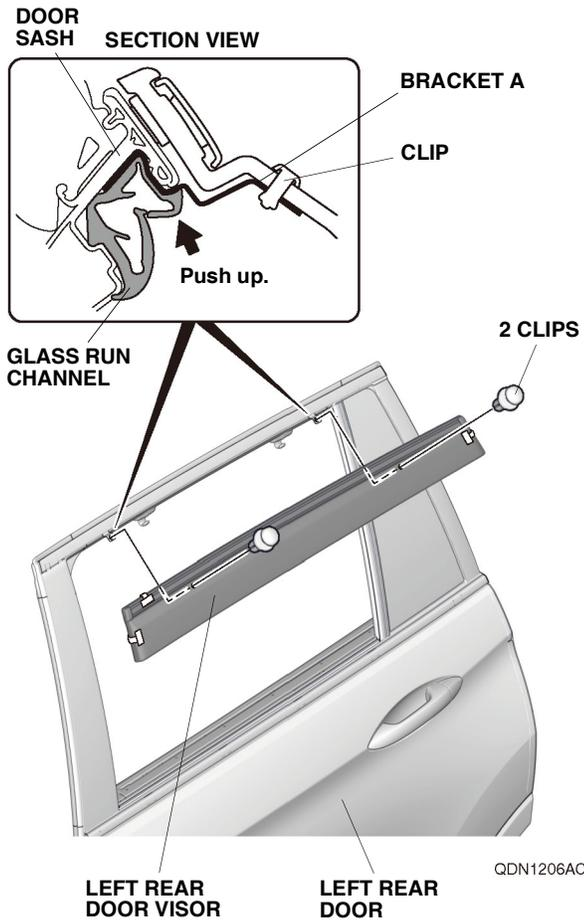
21. Using the two clips, secure the left rear door visor to the two brackets A as shown. Make sure to push up on the two brackets A while installing the two clips. NOTE: Be extremely careful when installing the clips; they cannot be reinstalled after installation.
