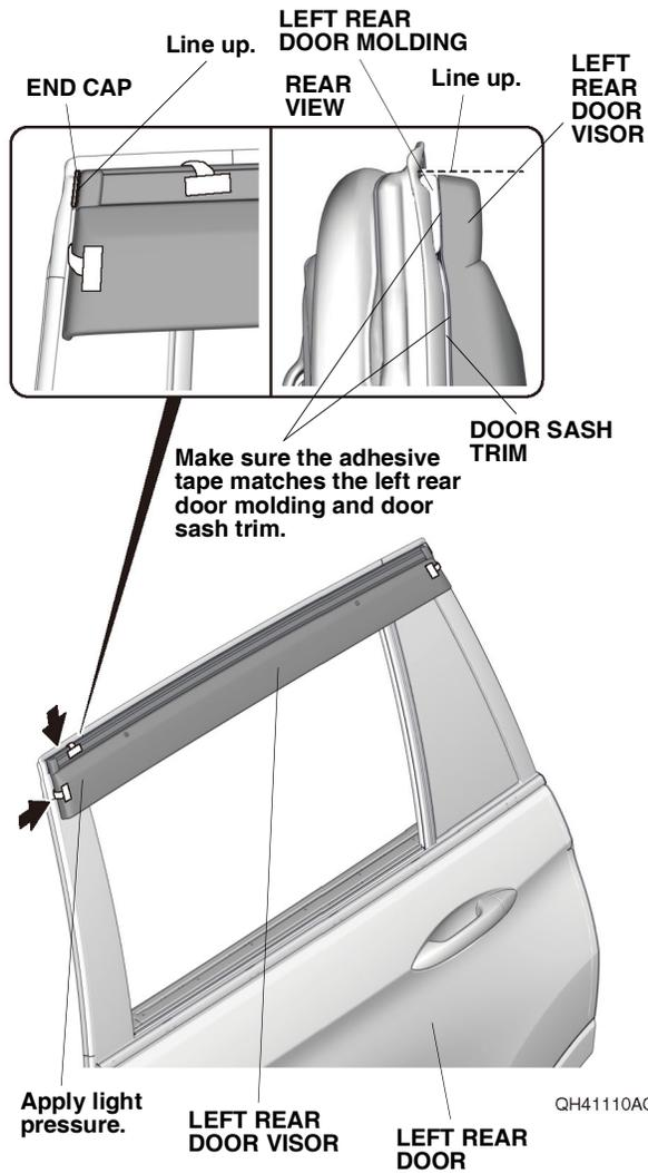
24. While applying light pressure against the left rear door visor, carefully remove the taped adhesive backing as shown. Make sure to push up on the two brackets A while removing the adhesive backing. NOTE: While removing the long top piece of adhesive backing, make sure that left rear door visor is positioned so that the top edge of vehicle chrome is hidden by left rear door visor.
