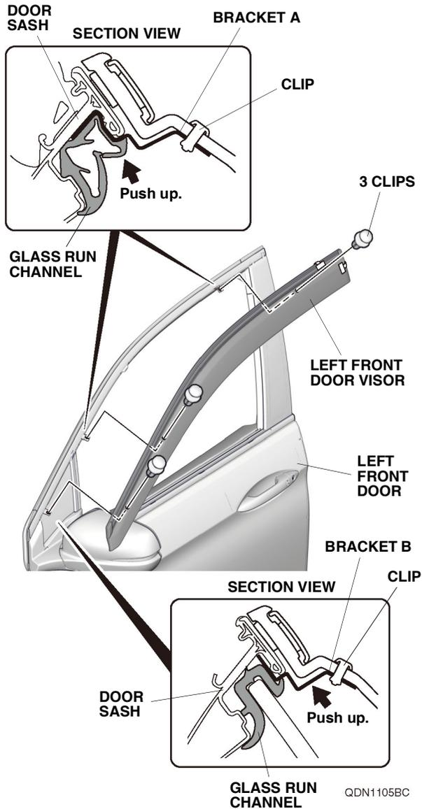
8. Using the three clips, secure the left front door visor to the two brackets A and one bracket B as shown. Make sure to push up on the two brackets A and one bracket B while installing three clips.
