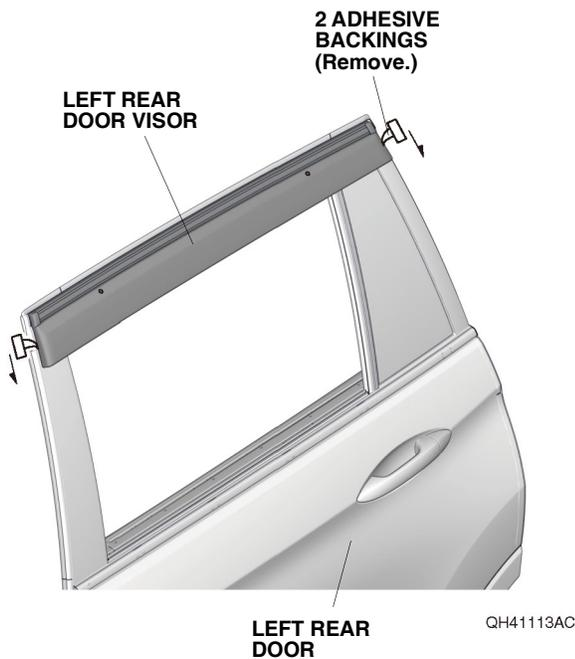
27. Using a rubber roller, apply firm pressure against the left rear door visor and roll from one end to the other.
