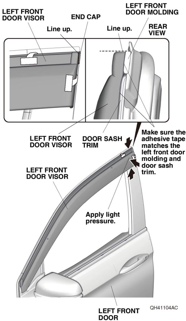
11. While applying light pressure against the left front door visor, carefully remove the taped adhesive backing as shown. Make sure to push up on the two brackets A and one bracket B while removing the adhesive backing.
