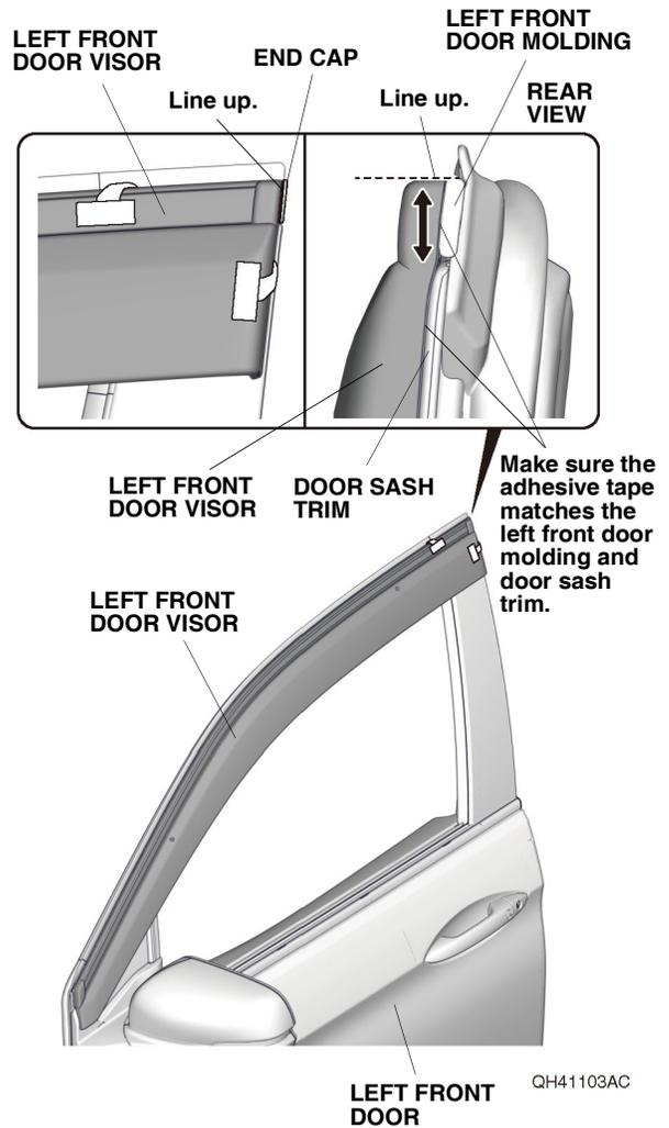
10. While lining up the left front door visor, apply light pressure against the left front door visor as shown.
