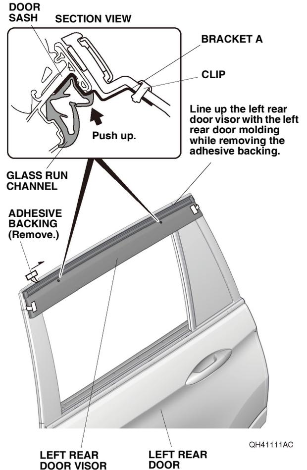
25. Using a rubber roller, apply firm pressure against the left rear door visor and roll from one end to the other.
