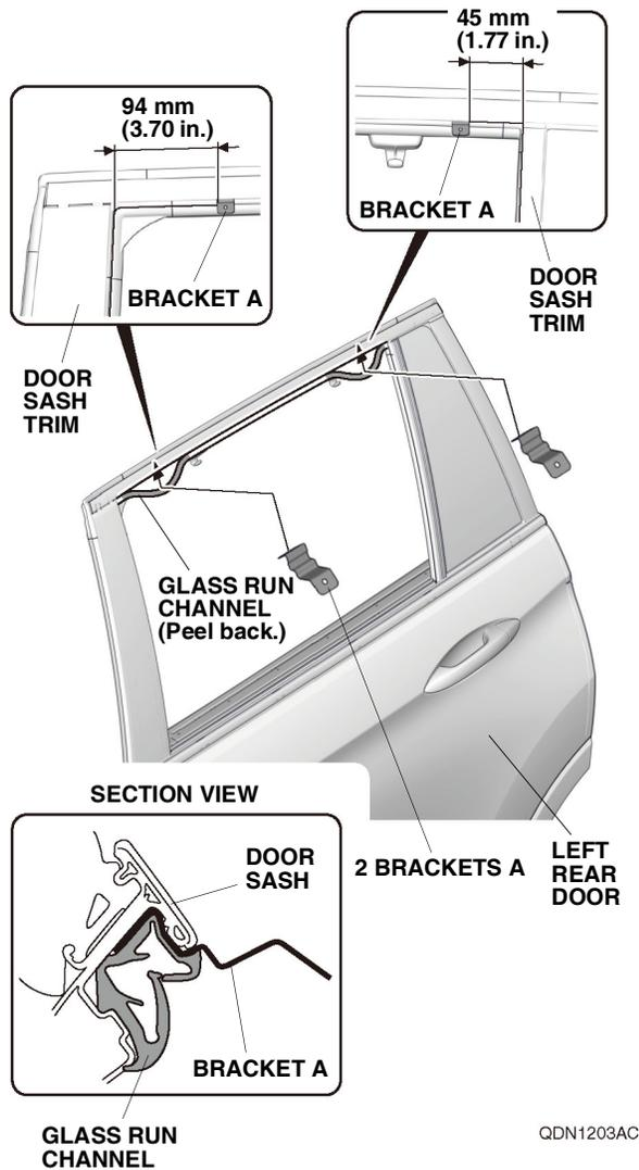
16. Peel back the glass run channel as shown.
