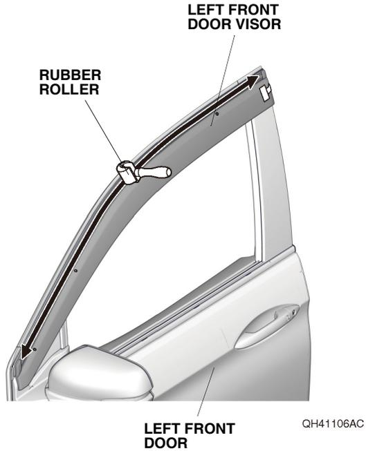
14. Using a rubber roller, apply firm pressure against the left front door visor and roll from one end to the other.
