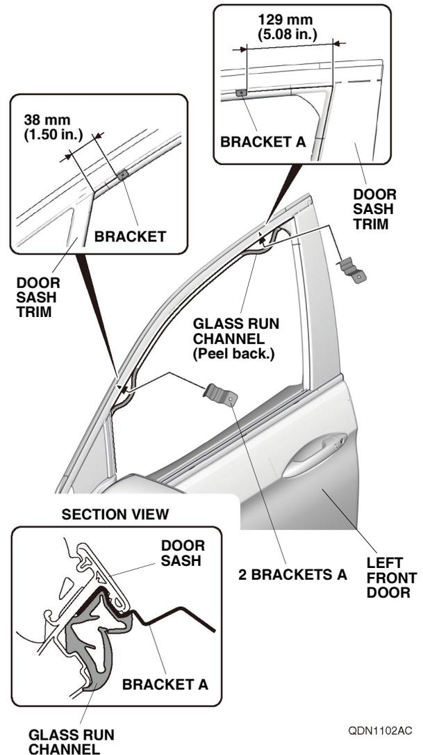
2. Peel back the glass run channel as shown.
