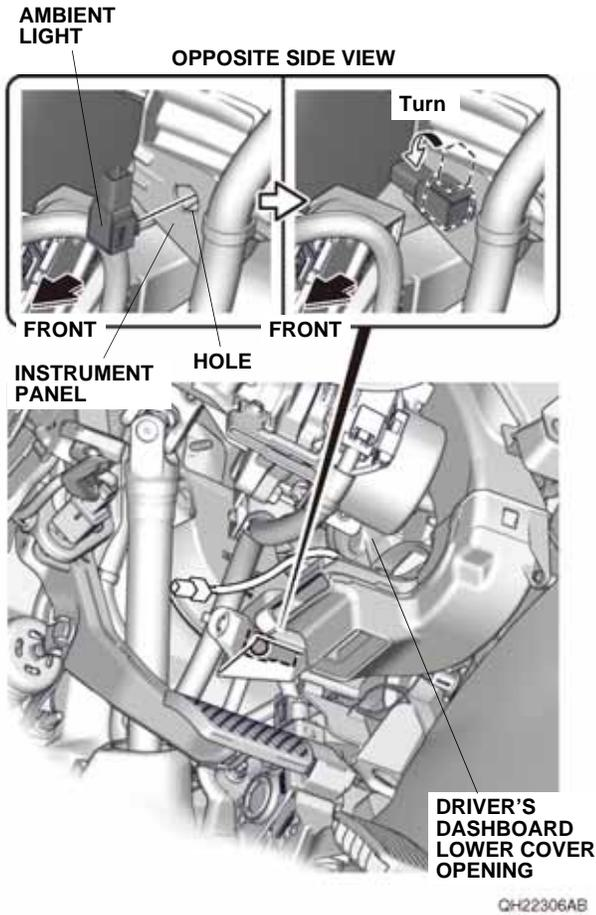
7. Plug the vehicle 2-pin connector into the ambient light.
