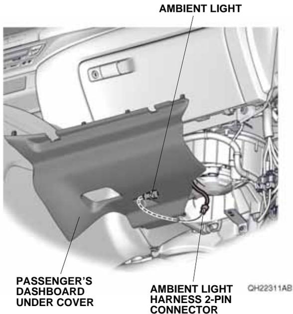
13. Check that all wire harnesses are routed properly and all connectors are plugged in.
