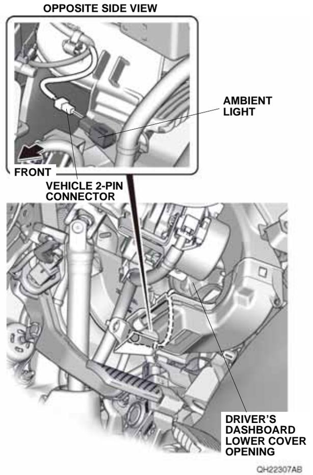
8. Install the ambient light to the passenger's dashboard under cover as shown.
